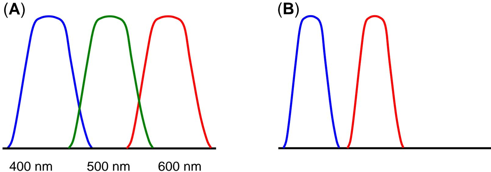
Spectral data of narrow-band imaging filters corresponding to red, green, and blue in comparison with that of standard filters. (a) Standard filters. (b) NBI filters. The center wavelengths of the dedicated trichromatic optical filters were shifted to shorter wavelengths.
